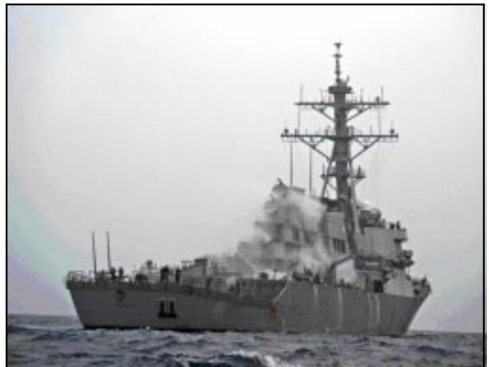
GULF OF ADEN The Arleigh Burke-class guided-missile destroyer USS Barry (DDG 52) conducts an operational check of the countermeasure wash down sprinkler system. The countermeasure wash down system washes the ships exterior in case of chemical, biological or radiological contamination.
